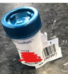
**One sticker only** - multiple labels stuck over the top of each other make the circumference of the pots too big for the multiprocessor, causing machine breakdowns, resulting in delay in processing & reporting.
